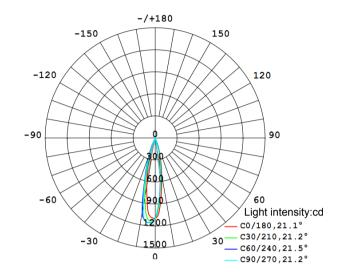
Mean beam angle (50%):21.2 °C
